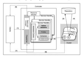
Fig. 2. Architecture overview. Dotted lines indicate asynchronous messages.
